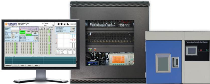
The custom Product Reliability Tester (PRT) is an Automated Test Equipment (ATE) system that provides a low cost, high performance, accelerated aging, burn-in, and qualification testing for laser diodes. The PRT uses precise control allowing the user to test up to 1024 laser diodes with various environmental chambers.
